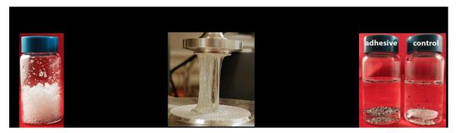
Repurposing sodium polyacrylate based superabsorbent to make pressure-sensitive adhesives followed by microplastics capture in aqueous media.
