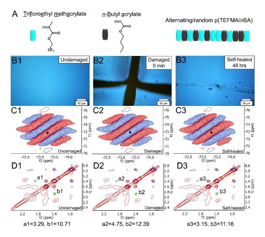
Chemical structure of 2,2,2-trifluoroethyl methacrylate (TFEMA) and n-butyl acrylate (nBA) as well as p(TFEMA/nBA) copolymers; (A) Optical images of p(TFEMA/nBA) copolymer films: undamaged (B1); damaged (B2) – cut size: ~50 µm; and self-healed (B3). 2D <sup>19</sup>F NOESY NMR spectra of undamaged (C1), damaged (C2) and self-healed (C3); 2D <sup>1</sup>H NOESY NMR spectra of undamaged (D1), damaged (D2) and self-healed (D3) copolymer
